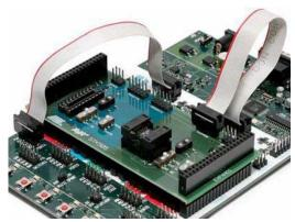
Figure 2-3: High voltage programming of the ATtiny24
