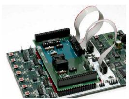
Figure 2-4: High voltage programming of the ATtiny26
