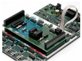
Figure 2-1: In-System Programming of the ATtiny24
