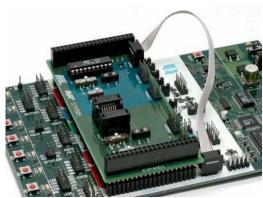
Figure 2-2: In-System Programming of the ATtiny26
