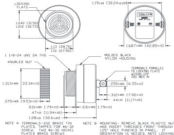
NOTE A: TERMINALS-032 BRASS TIN PLATED, TAPPED FOR #6-32 SCREW. TWO #6-32 NICKEL PLATED BRASS SCREWS INCLUBED. WILL ACCEPT 1/4\* OUICK CONNECT.
