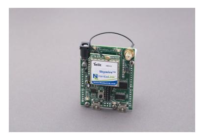
A properly mounted Skywire™ Modem with U.FL cable attached to top U.FL connector X1
