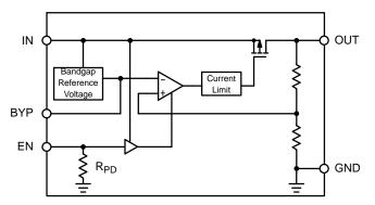
Figure 2. Simplified Block Diagram
