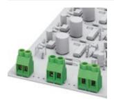
PCB terminal block, Nominal current: 32 A, Nom. voltage: 630 V, Pitch: 7.62 mm, Number of positions: 9, Connection method: Screw connection, Mounting: Soldering, Conductor/PCB connection direction: 0 °, Color: Pebble gray, The article can be aligned to create different nos. of positions!
