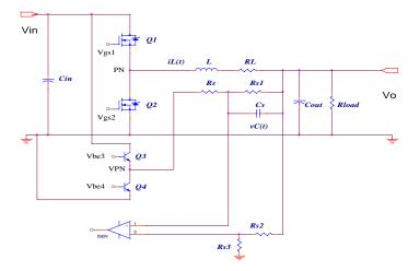
Fig.3 Current limit scaling.
