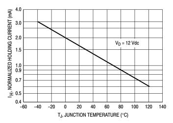
Figure 5. Typical Holding Current versus Temperature
