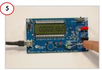
Touch thermocouple and monitor voltage displayed on LCD.
