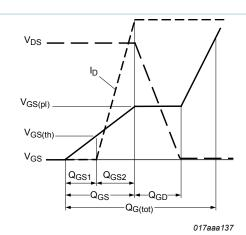
Fig. 15. Gate charge waveform definitions
