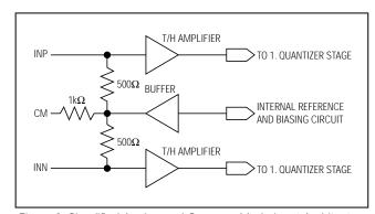
Figure 2. Simplified Analog and Common-Mode Input Architecture
