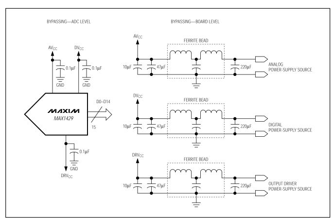
Figure 9. Grounding, Bypassing, and Decoupling Recommendations for MAX1429
