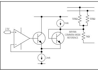
Figure 3. Simplified Reference Architecture
