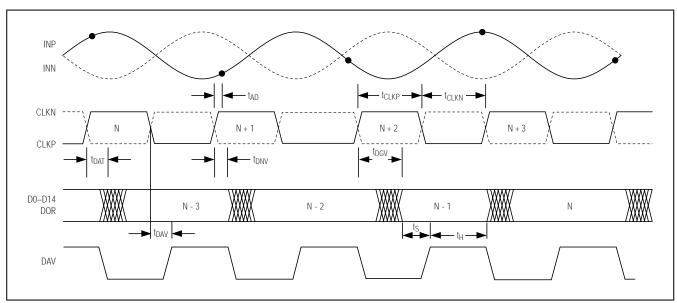
Figure 4. System and Output Timing Diagram
