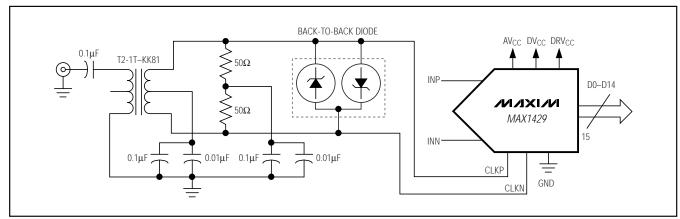
Figure 5. Transformer-Coupled Clock Input Configuration
