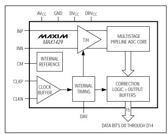
Figure 1. Simplified MAX1429 Diagram
