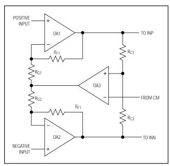
Figure 8. DC-Coupled Analog Input Configuration
