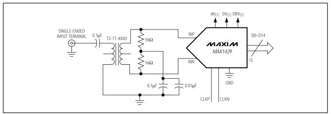
Figure 6. Transformer-Coupled Analog Input Configuration
