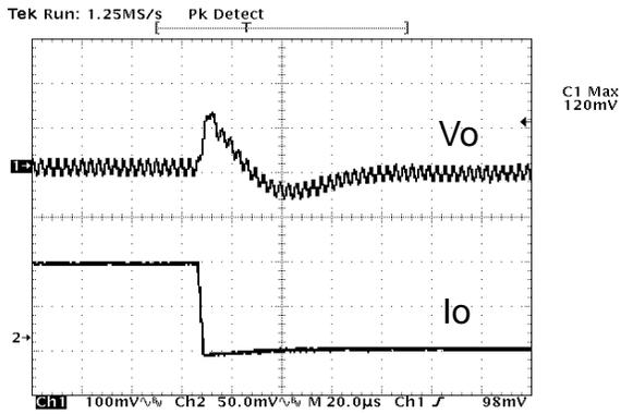
**Figure 24:** Typical transient response to step load change at  $5A/\mu S$  from 100% to 50% of  $I_o$ , max at  $12V_{in}$ ,  $5.0V$  out ( $C_{out} = 1\mu F + 100\mu F$  ceramic,  $470\mu F$  poscap).
