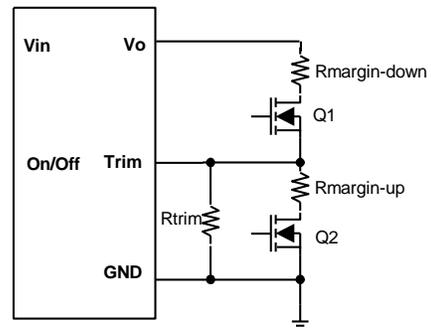
**Figure 36:** Circuit configuration for output voltage margining
