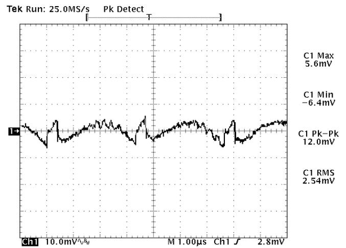
**Figure 11:** Output ripple & noise at 12Vin, 1.2V/20A out.
