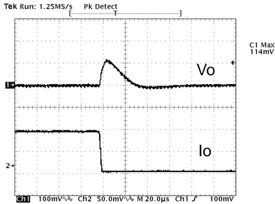
**Figure 20:** Typical transient response to step load change at  $5A/\mu S$  from 100% to 50% of  $I_o$ , max at  $12V_{in}$ ,  $1.2V$  out ( $C_{out} = 1\mu F + 100\mu F$  ceramic,  $470\mu F$  poscap).
