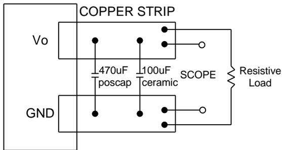
Note: Use a 470µF poscap and 100µF ceramic. Scope measurement should be made using a BNC connector.
