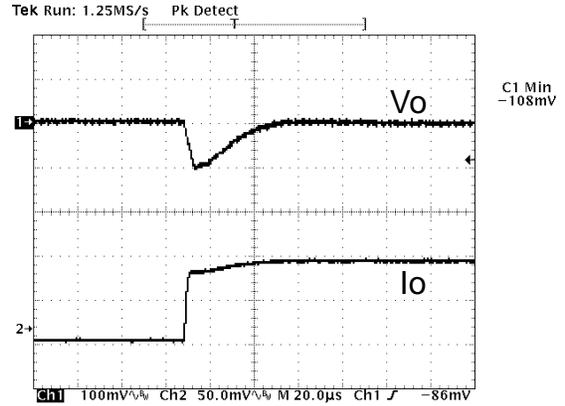
**Figure 19:** Typical transient response to step load change at  $5A/\mu S$  from 50% to 100% of  $I_o$ , max at  $12V_{in}$ ,  $0.75V$  out ( $C_{out} = 1\mu F + 100\mu F$  ceramic,  $470\mu F$  poscap).
