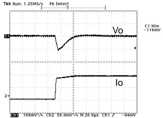
**Figure 21:** Typical transient response to step load change at  $5A/\mu S$  from 100% to 50% of  $I_o$ , max at  $12V_{in}$ ,  $1.2V$  out ( $C_{out} = 1\mu F + 100\mu F$  ceramic,  $470\mu F$  poscap).
