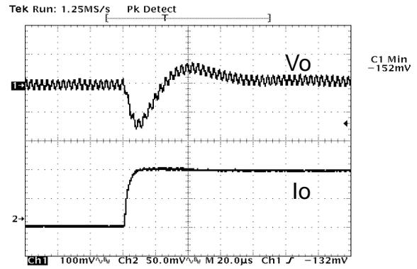
**Figure 25:** Typical transient response to step load change at  $5A/\mu S$  from 100% to 50% of  $I_o$ , max at  $12V_{in}$ ,  $5.0V$  out ( $C_{out} = 1\mu F + 100\mu F$  ceramic,  $470\mu F$  poscap).
