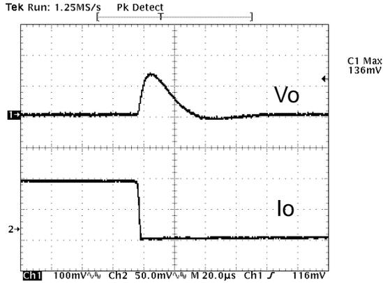
**Figure 18:** Typical transient response to step load change at  $5A/\mu S$  from 100% to 50% of  $I_o$ , max at  $12V_{in}$ ,  $0.75V$  out ( $C_{out} = 1\mu F + 100\mu F$  ceramic,  $470\mu F$  poscap).
