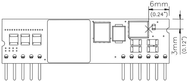
**Figure 41:** Temperature measurement location
