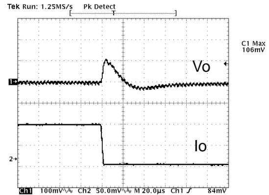
**Figure 22:** Typical transient response to step load change at  $5A/\mu S$  from 100% to 50% of  $I_o$ , max at  $12V_{in}$ ,  $2.5V$  out ( $C_{out} = 1\mu F + 100\mu F$  ceramic,  $470\mu F$  poscap).
