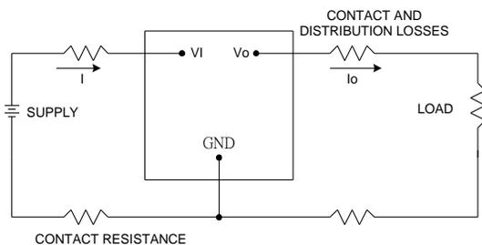
**Figure 30:** Output voltage and efficiency measurement test setup
