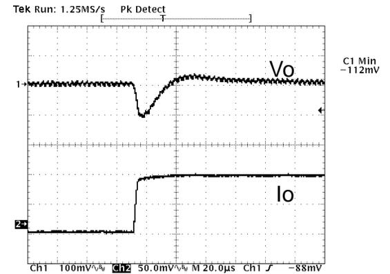
**Figure 23:** Typical transient response to step load change at  $5A/\mu S$  from 50% to 100% of  $I_o$ , max at  $12V_{in}$ ,  $2.5V$  out ( $C_{out} = 1\mu F + 100\mu F$  ceramic,  $470\mu F$  poscap).
