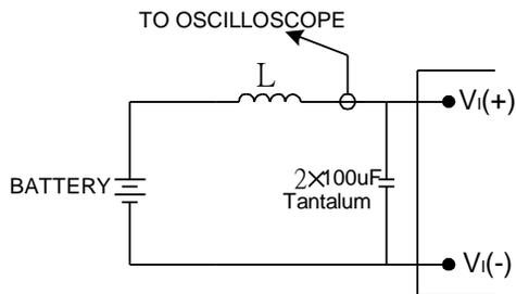
Note: Input reflected-ripple current is measured with a simulated source inductance. Current is measured at the input of the module.
