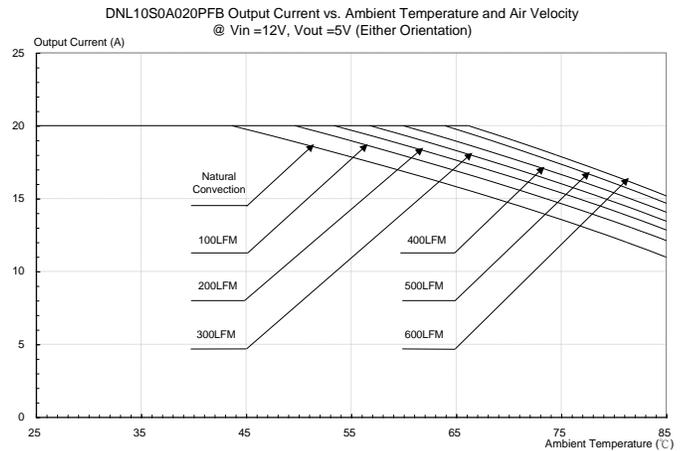
**Figure 45:** Output current vs. ambient temperature and air velocity @ Vin=12V, Vout=5.0V(Either Orientation)
