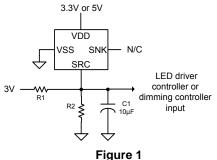
The example in figure one shows a fully automatic lighting control solution with no user interaction. Choose R1 and R2 values for any desired minimum brightness and slope. Choose C1 to adjust response time. As an example, let's say you wish to generate an output voltage from 0.25V to 1.25V to drive the input of an LED driver controller. The 0.25V represents the minimum LED brightness and 1.25V represent the maximum. The first step would be to determine the ratio of R1 and R2.
