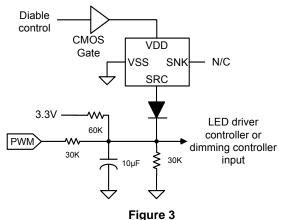
The preceding examples represent just a few of the many ways the sensor can be used. For example since there is also a complimentary sink output a resistor from VDD to SNK could develop a voltage that could be compared (with some hysteresis) to a fixed (or adjustable) reference voltage and develop a logic signal. In the case of street lighting or operation of shades such a signal would engage the function when reaching the correct ambient light level.
