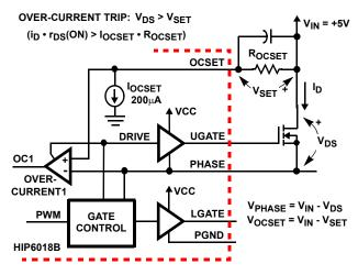
FIGURE 9. OVER-CURRENT DETECTION
