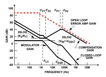
FIGURE 12. ASYMPTOTIC BODE PLOT OF CONVERTER GAIN
