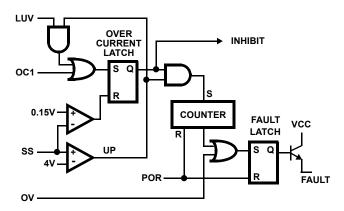
FIGURE 7. FAULT LOGIC - SIMPLIFIED SCHEMATIC
