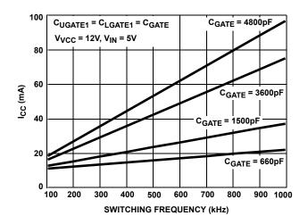
FIGURE 5. BIAS SUPPLY CURRENT vs FREQUENCY
