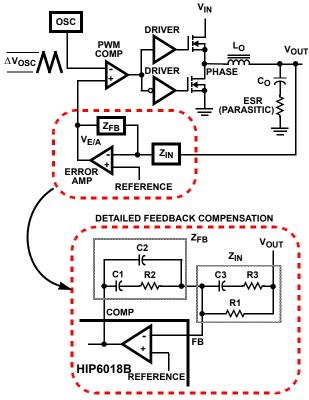
FIGURE 11. VOLTAGE-MODE BUCK CONVERTER COMPENSATION DESIGN
