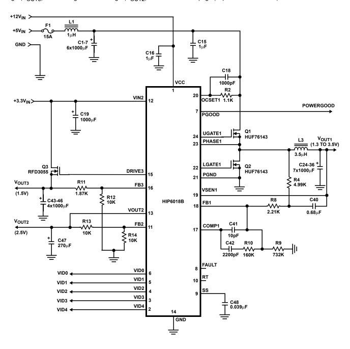
FIGURE 15. APPLICATION CIRCUIT
