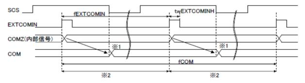
1:LC inversion polarity has been set by the rising timing of EXTCOMIN in internal circuit block as COMZ signal, 2: The period of EXTCOMIN should be constant.
