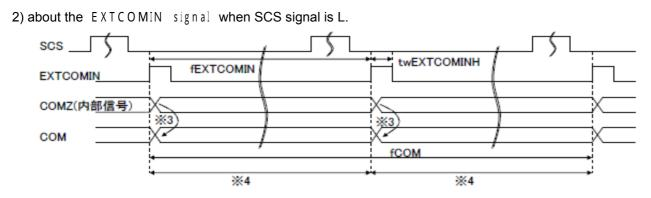
3:LC inversion polarity has been set by the rising timing of EXTCOMIN in internal circuit block as COMZ signal, 4: The period of EXTCOMIN should be constant.
