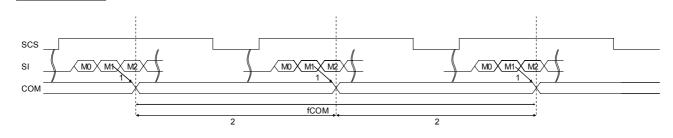
M1:LC polarity inversion flag: If M1is "H" then VCOM="H" is output. If M1 is "L" then VCOM="L" is output.
