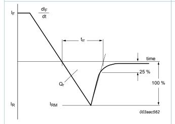
Fig. 6. Reverse recovery definitions; ramp recovery
