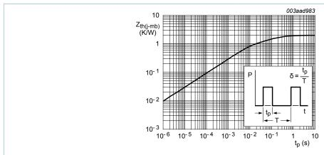
Fig. 3. Transient thermal impedance from junction to mounting base as a function of pulse width
