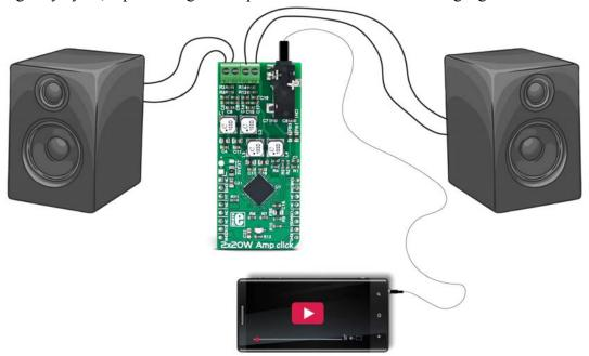
The output of the modulator is used to gate the output transistors on and off, alternately. The high efficiency of a Class D amplifier is due to the switching operation of the output stage transistors. Since the transistors are either fully ON or fully OFF, they spend a small amount of time in the linear region and consume little amounts of power.
