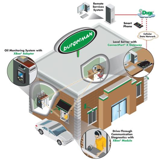
In the diagram above, a Digi ConnectPort X2 gateway is used to connect an RF network (plus other peripherals) to the Internet via either the Ethernet port or a cellular WAN connection. Note that gateways are programmable and can also be used to run local applications, which can monitor/control the RF network, with or without Internet connectivity.
