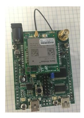
A properly mounted Skywire NL-SW-LTE-S7xxx modem with U.FL cable attached to top U.FL connector X1
