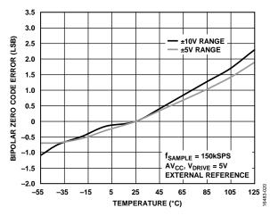
Figure 8. Bipolar Zero Code Error vs. Temperature
