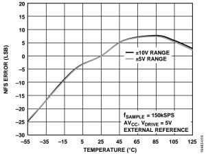
Figure 5. NFS Error vs. Temperature
