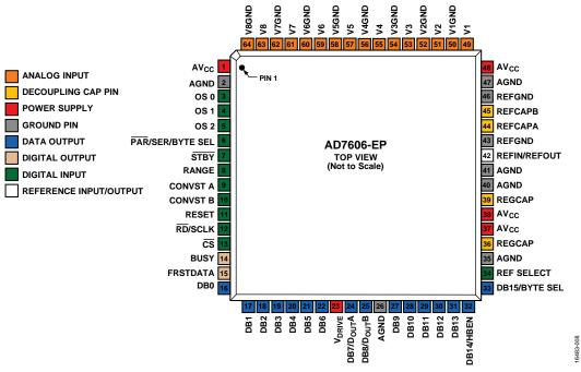
Figure 4. Pin Configuration
