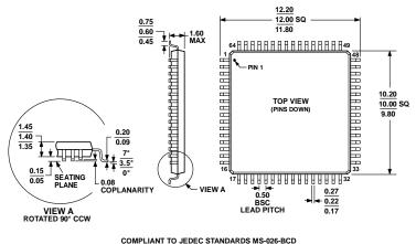
Figure 12. 64-Lead Low Profile Quad Flat Package [LQFP] (ST-64-2) Dimensions shown in millimeters
