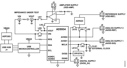
Figure 1. AD5934 Evaluation Board Block Diagram
