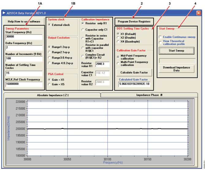
Figure 14. AD5934 Evaluation Software Main Dialog Box (The Impedance Profile of a 200 k $\Omega$  Resistor Is Displayed.)
