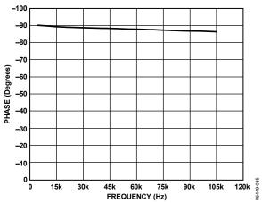
Figure 35. Phase Response of a Capacitor
