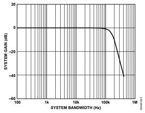
Figure 33. Typical AD5934 System Bandwidth
