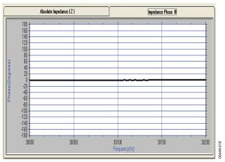
Figure 19. The **Impedance Phase Ø** Tab on the Main Dialog Box (the Phase of a 200 kΩ Resistor (0°) Is Displayed)
