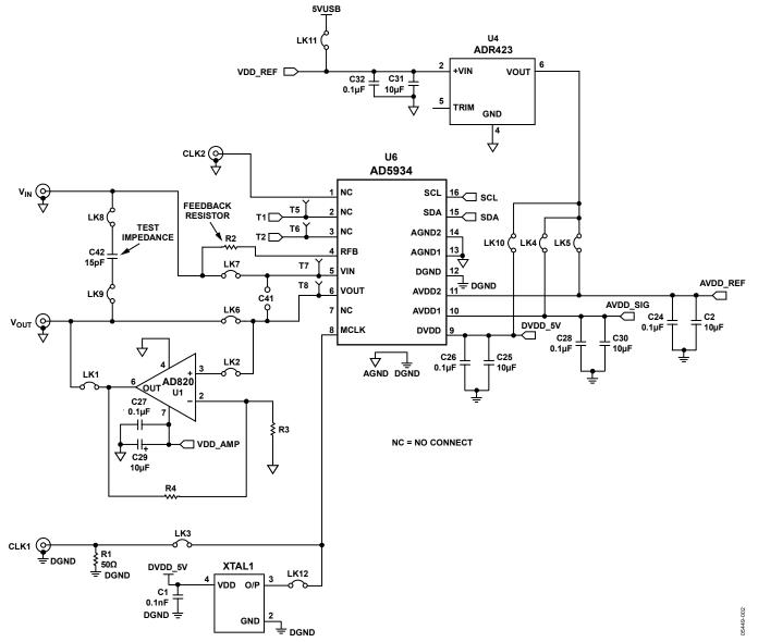
Figure 2. Setup Link Position Circuit (A 15 pF Capacitor Connected Between VIN and VOUT, with RFB =  $200 \, \mathrm{k}\Omega$  and a Precision 16 MHz Crystal Connected to MCLK)
