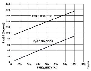
Figure 34. System Phase Response vs. Capacitive Phase
