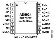
Figure 3. Pin Configuration
