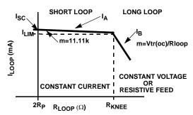
FIGURE 3. I<sub>LOOP</sub> vs. R<sub>LOOP</sub> LOAD CHARACTERISTIC
