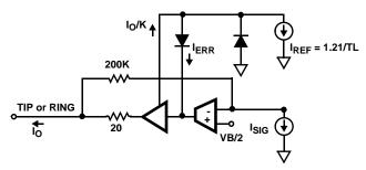
FIGURE 1. CURRENT LIMIT FUNCTIONAL DIAGRAM
