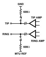
FIGURE 8. LPS 2-WIRE INTERFACE CIRCUIT DIAGRAM
