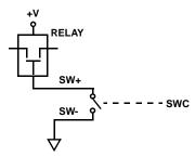
FIGURE 15. EXTERNAL RELAY SWITCHING
