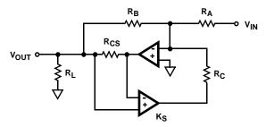
FIGURE 9. VOLTAGE FEED CURRENT SENSE DIAGRAM
