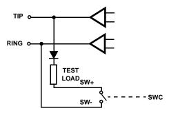
FIGURE 16. TEST LOAD SWITCHING
