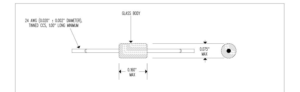
RESISTANCE @  $+25^{\circ}C = 30,000 \Omega \pm 10\%$ RESISTANCE/TEMPERATURE CURVE = "H" TEMPERATURE COEFFICIENT @  $+25^{\circ}C = -4.29\%$ /°C NOMINAL BETA " $\beta$ " (0 TO  $+50^{\circ}C$ ) = 3,810°K NOMINAL DISSIPATION CONSTANT = 2 mW/°C NOMINAL (STILL AIR) THERMAL TIME CONSTANT = 5 SECONDS NOMINAL (STILL AIR) THERMAL TIME CONSTANT = 0.5 SECONDS NOMINAL (STIRRED OIL) MAXIMUM TEMPERATURE RATING =  $+300^{\circ}C$
