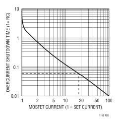
Figure 2. Shutdown Time vs MOSFET Current
