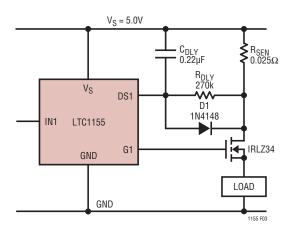
Figure 3. Using a Speed-Up Diode
