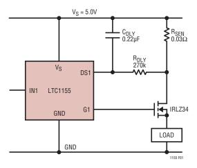
Figure 1. Adding an RC Delay
