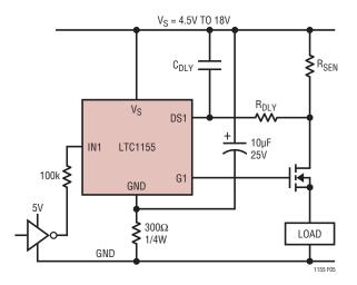
Figure 5. Reverse Battery Protection
