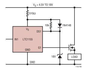
Figure 6. Overvoltage Shutdown and Protection
