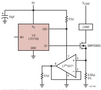
\*DO NOT SUBSTITUTE. MUST BE A PRECISION, SINGLE SUPPLY, MICROPOWER OP AMP (I  $_{\textrm{Q}} < 60 \mu \textrm{A})$
