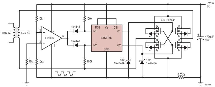
MOSFETS ARE SYNCHRONOUSLY ENHANCED WHEN RECTIFIER CURRENT EXCEEDS 300mA \*NO HEATSINK REQUIRED \*\*INTERNAL BODY DIODE OF MOSFET
