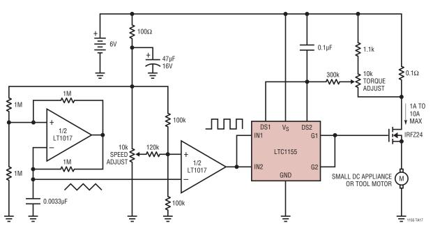
SPEED IS PROPORTIONAL TO PULSE WIDTH. TORQUE IS PROPORTIONAL TO CURRENT
