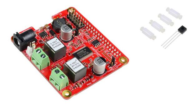
The JustBoom Amp HAT is a high-quality audio amplifier designed specifically for the Raspberry Pi. Digital-to-analog conversion is also included with the Amp HAT, so no external sound cards or DACs are required. Simply stack the plug-and-play add-on board (HAT) onto your Raspberry Pi A+, B+, 2B or the new 3B, and it will be ready to use immediately.
