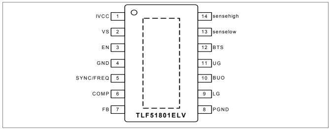
Figure 2 Pin Configuration
