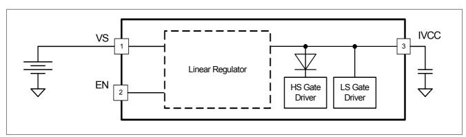
Figure 11 Linear Regulator Block Diagram and Simplified Application Circuit
