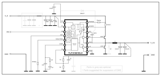
Figure 13 Application Diagram (Current limitation with Shunt-configuration)
