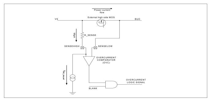
Figure 8 Rdson-configuration for current limitation
