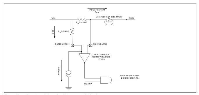
Figure 9 Shunt-configuration for current limitation
