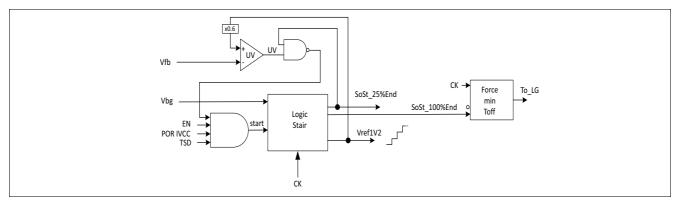
Figure 4 Soft start block diagram
