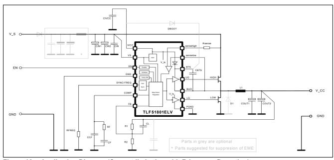
Figure 12 Application Diagram (Current limitation with Rdson-configuration)
