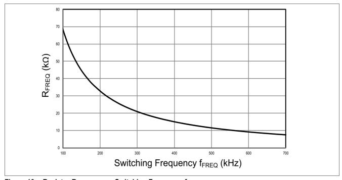
Figure 10 Resistor R<sub>FREQ</sub> versus Switching Frequency f<sub>FREQ</sub>
