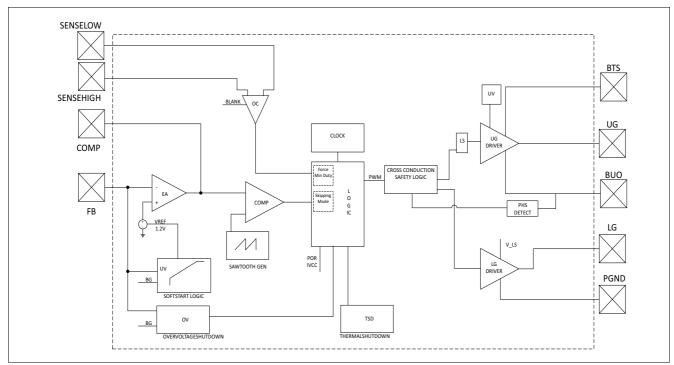
Figure 3 Block Diagram Buck Regulator
