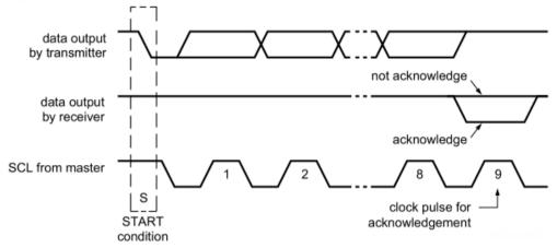
Figure 10. Acknowledgment on I2C Bus
