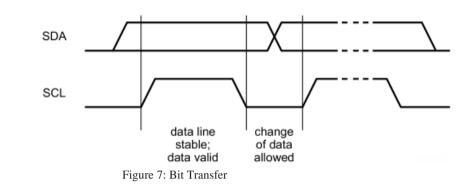
Both data and clock lines remain HIGH when the bus is not busy. A HIGH-to-LOW transition of the data line while the clock is HIGH is defined as the START condition (S). A LOW-to-HIGH transition of the data line while the clock is HIGH is defined as the STOP condition (P)
