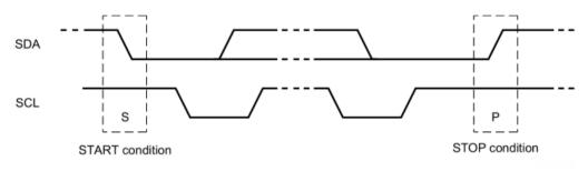
Figure 8. Definition of Start and Stop Conditions
