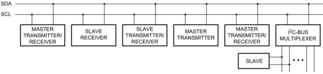
Figure 9. System Configuration
