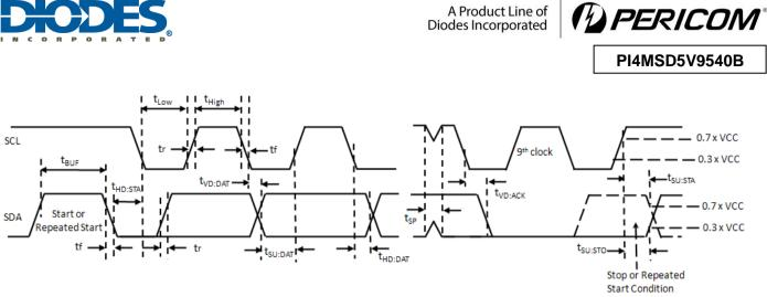
Figure 2. Definition of timing on the I2C-bus
