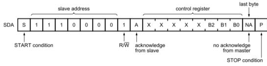
Figure 12. Read Control Register
