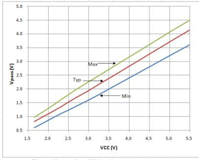
Figure 6:Vpass voltage VS Vcc
