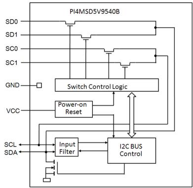
Figure 1: Block Diagram
