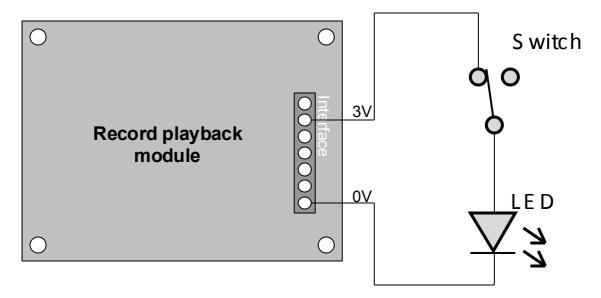
When connecting the LED make sure that the flat edge / short lead is connected to the OV connection on the interface connector. The switch should be connected to the 3V connection.
