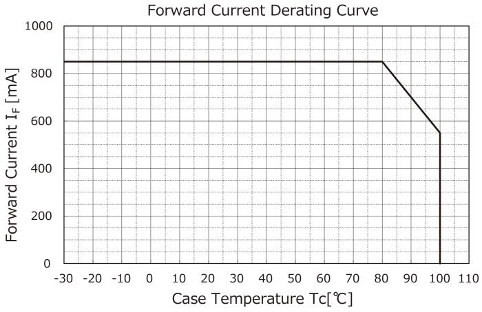
(Note) To keep the case temperature lower than the rating, enough heat-radiation performance needs to be secured by using an adequate heat sink (refer to section 7-③).
