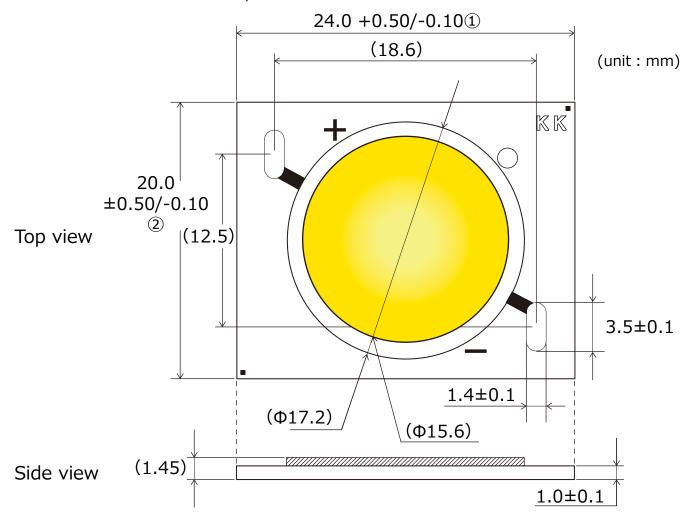
Values inside parentheses are reference values. External sizes of 1, 2 are determined by maximum dimensions, that include salient areas on the edges of respective sides.
