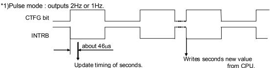
In a pulse mode, update of seconds is behind with about  $46\mu s$  from a falling edge of INT.
