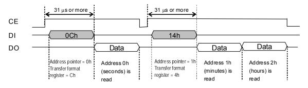
Incorrect example 2: If interval is less than 31 µs when time write operation is started
