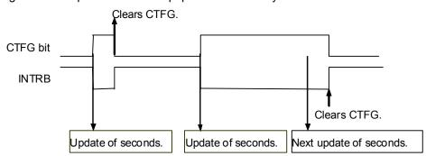
Note: When Clock Precision Adjustment Function works, a period of interrupt changes by that quantity of the adjustment once per 20 seconds or one minute.
