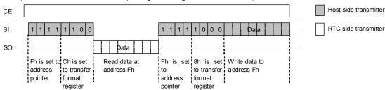
\* The following table provides a summary of the relation between the read/write format and settings in the transfer format register.
