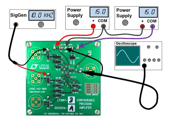
Figure 1. Proper Evaluation Equipment Setup
