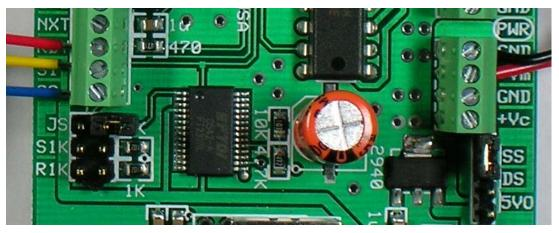
(note that the JS jumper is positioned so that only one pin is connected to the jumper; this allows you to not lose the jumper....)
