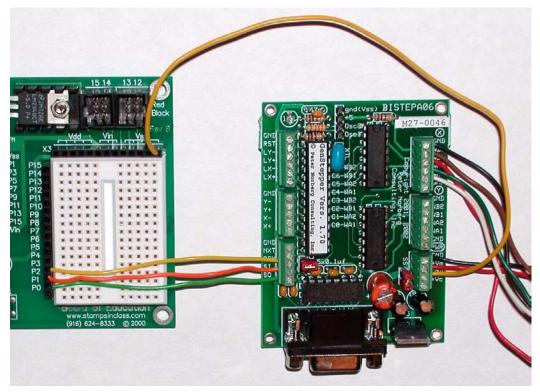
Observe that the ground between the boards is accomplished by a wire from the extra "GND" connector on the BiStepA06 power connector (lower right of board as shown) to one of the "Vss" signals on the BOE.
