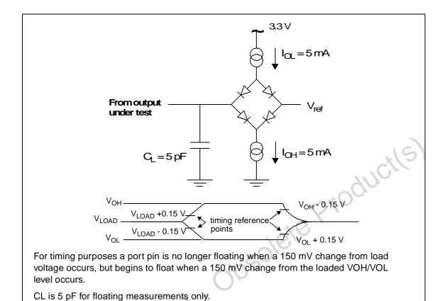
Figure 10 Float waveforms
