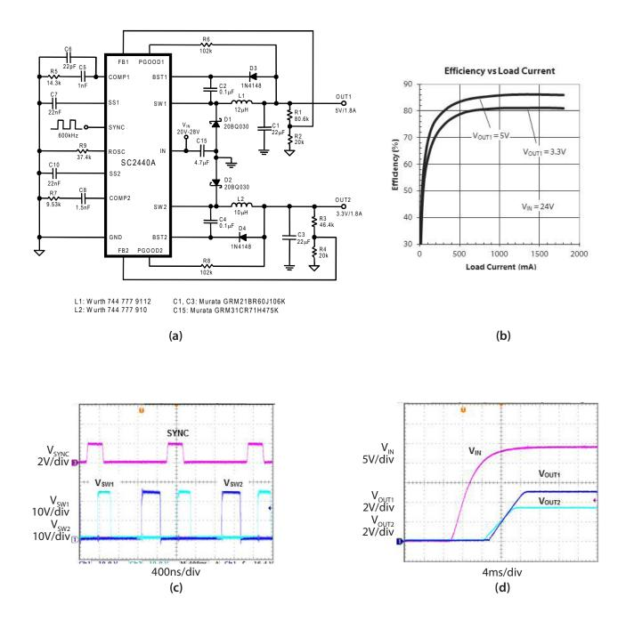
Figure 15. (a) Synchronized 600kHz 24V to 5V and 3.3V Dual Step-down Converter. The free-running frequency of the regulator is set to 580kHz.
