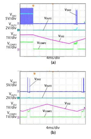
Figure 9. Overload Hiccup of the 5V Output Channel in Figure 1.
