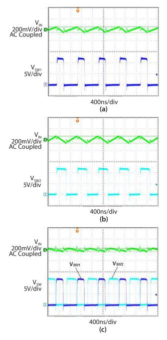
Figure 6. Input Voltage Ripple Generated by the DC-DC Converter in Figure 1.
