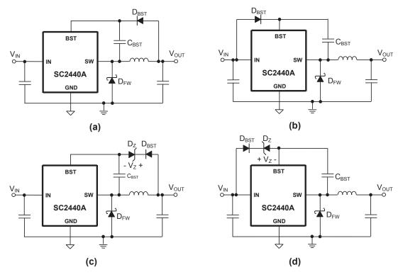
Figure 7(a)-(d). Bootstrap Configurations for the SC2440A
