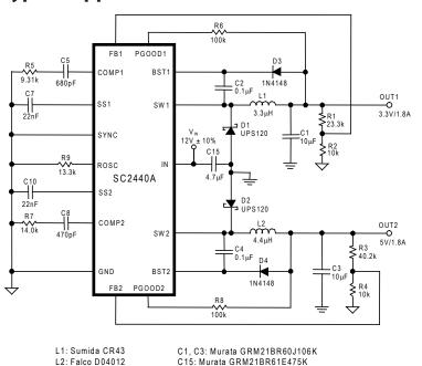
Figure 1. 1.3MHz 12V to 5V and 3.3V Step-down Converter
