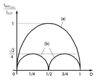
Figure 5. Normalized C<sub>IN</sub> RMS Ripple Current as a Function of the Duty Cycle D for the Following Regulators:
