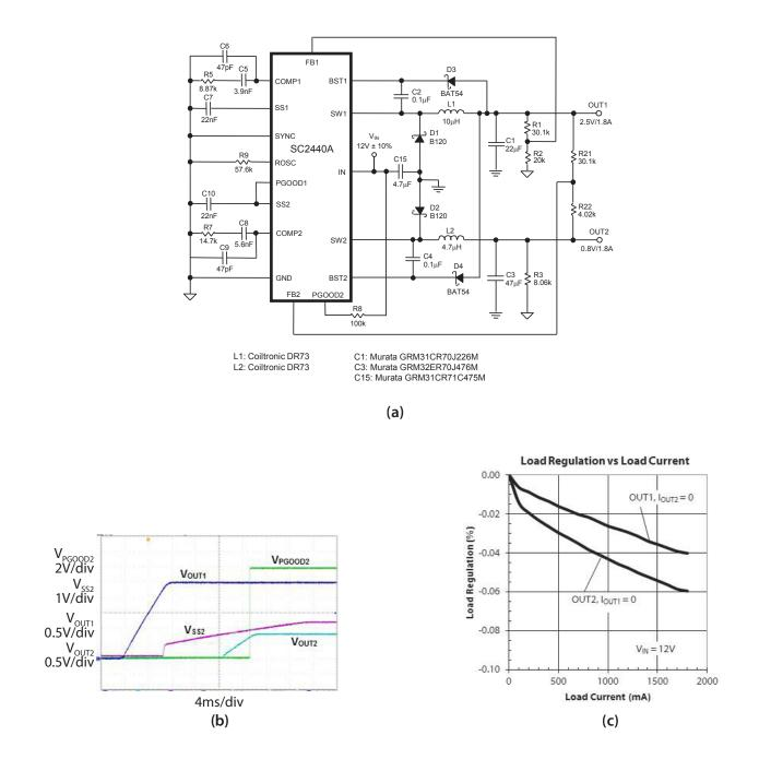
Figure 16. Stepping Down to a Voltage Lower Than the Feedback Voltage. (a) 400kHz 12V to 2.5V and 0.8V Step-down Converter. R<sub>3</sub> is a pre-load to shunt the current from R<sub>21</sub> and R<sub>22</sub> before PGOOD1 releases SS2. (b) Start-up waveform ( $I_{OUT1} = I_{OUT2} = 1A$ ). (c) Channel 2 load regulation is slightly below that of channel 1 because V<sub>FB2</sub> is derived from V<sub>OUT1</sub>.
