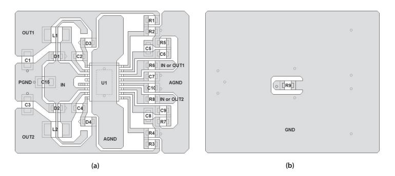
Figure 14. Suggested PCB Layout for the SC2440A (a) Top Layer and (b) Bottom Layer
