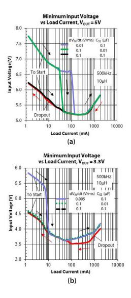
Figure 8. The Minimum Input Voltage to Start and to Run Before Dropout. The regulator is bootstrapped from its output [Figure 7(a)] with 1N4148. The minimum starting  $V_{IN}$ decreases when  $C_{SS}$  or  $dV_{IN}/dt$  increases. (a)  $V_{OUT} = 5V$ (b)  $V_{OUT} = 3.3V$
