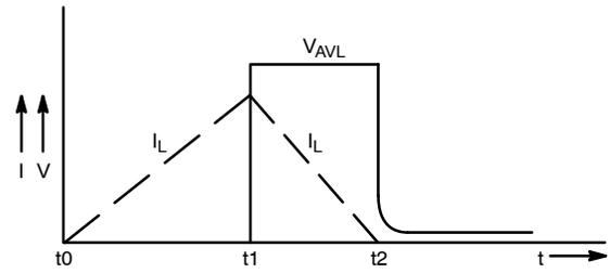
Figure 9. Unclamped Inductive Switching Test Circuit & Waveform
