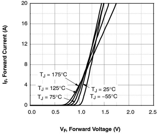
Figure 1. Forward Characteristics
