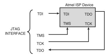
**Note:** You will need to reserve space on your circuit board to accommodate a 10-pin male header for the JTAG interface. The pinout for this header must match the Atmel-ISP cable connector pinout. The JTAG interface pins for each Atmel device must also be connected to this header.
