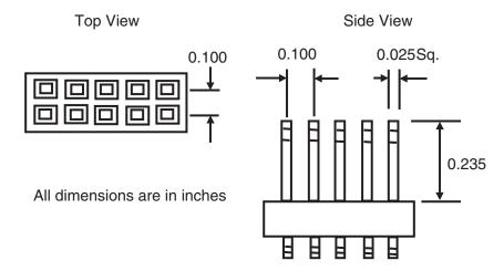
Figure 4-8. 10-pin Male Header Pinout
