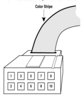
**Note:** Your circuit board must supply  $V_{\text{CC}}$  and GND to the Atmel-ISP cable through the 10-pin male header.
