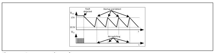
Figure 35 **Brown out mode waveform**
