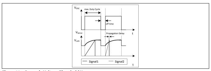
Figure 22 Dynamic Voltage Threshold V<sub>csth</sub>
