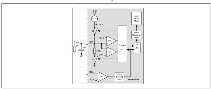
Figure 23 Basic and Extendable Blanking Mode
