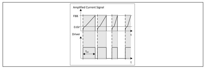
Figure 6 Pulse Width Modulation
