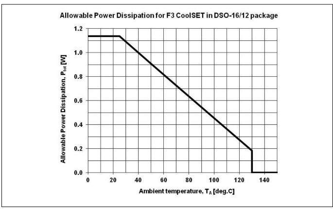
Figure 38 Power dissipation; Ptot=f(Ta)
