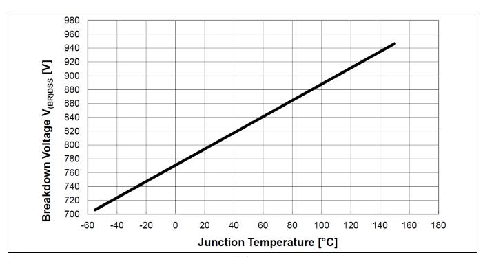
Figure 39 Drain-source breakdown voltage;  $V_{BR(DSS)}=f(T_j)$ ,  $I_D=0.25mA$
