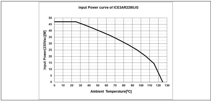
Input power curve V<sub>IN</sub>=230 V<sub>AC</sub>; P<sub>in</sub>=f(T<sub>a</sub>) Figure 41
