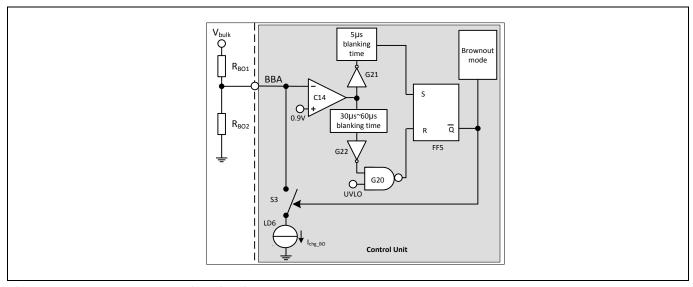
Figure 34 Brown out detection circuit
