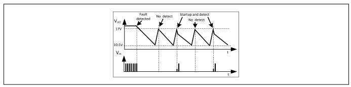
Figure 30 Odd skip auto restart waveform
