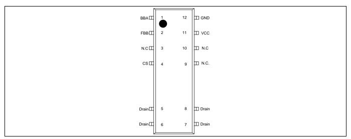
Figure 2 Pin configuration PG-DSO-12(top view)
