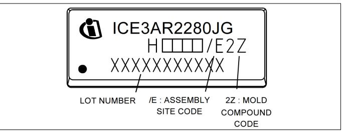
Figure 43 Marking for ICE3AR2280JG
