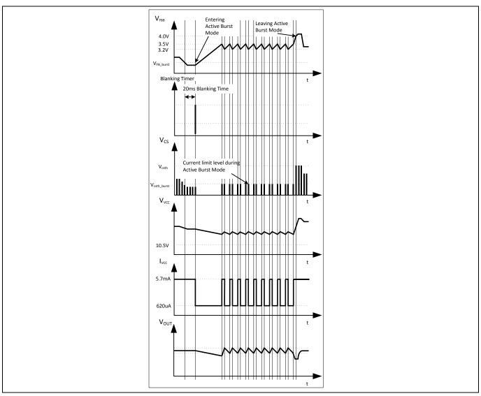
Figure 27 Signals in Active Burst Mode
