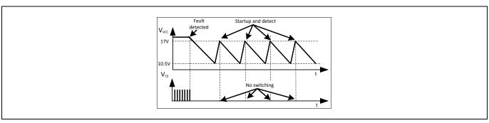
Figure 29 Non switch auto restart waveform
