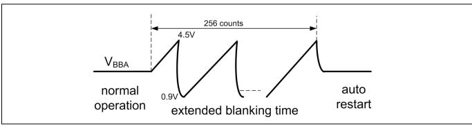
Waveform at extended blanking time Figure 24
