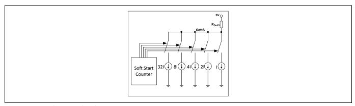
Figure 12 Soft Start Circuit
