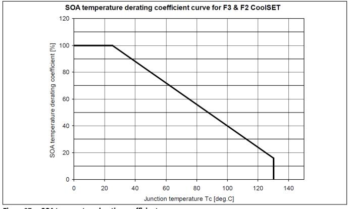
Figure 37 SOA temperature derating coefficient curve
