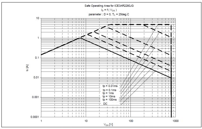
Figure 36 Safe Operating Area (SOA) curve for ICE3AR2280JG
