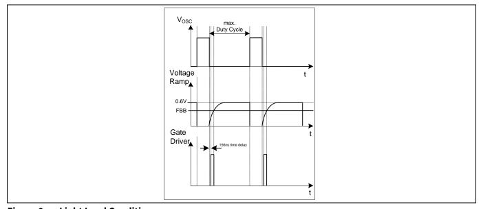
Figure 8 **Light Load Conditions**
