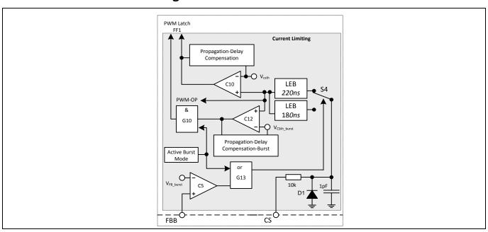
Figure 18 Current Limiting Block
