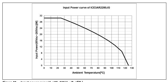
Figure 40 Input power curve  $V_{IN}=85\sim265 V_{AC}$ ;  $P_{in}=f(T_a)$
