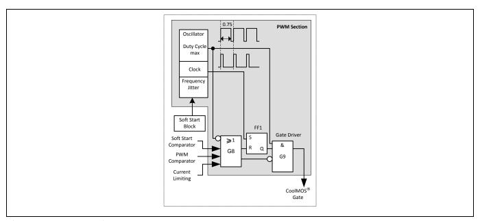
Figure 15 PWM Section Block
