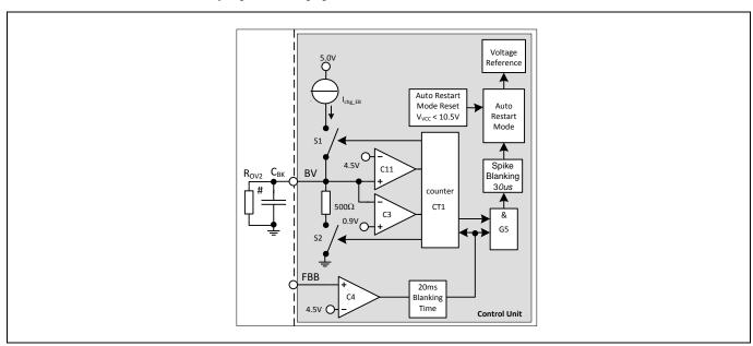
Figure 33 Over load, open loop protection
