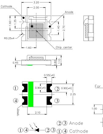
For reflow soldering (propose)
