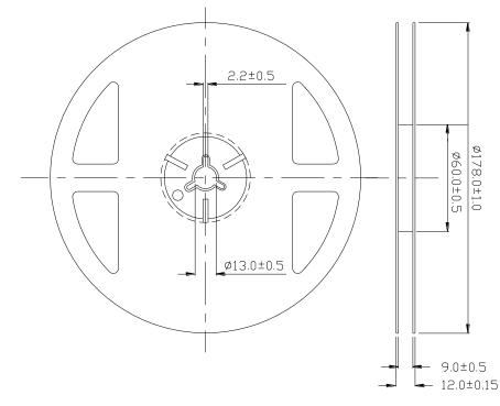
**Note:** The tolerances unless mentioned is  $\pm 0.1$ mm ,Unit = mm **2. Carrier Tape Dimensions:(Quantity: 3000pcs/reel)**
