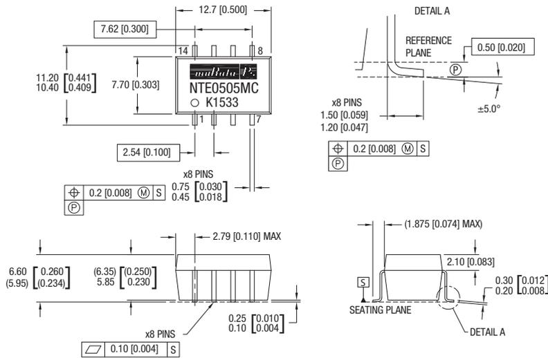
All dimensions in mm  $\pm 0.25$ mm (inches  $\pm 0.01$ ). All pins on a 2.54 (0.1) pitch and within  $\pm 0.25$  (0.01) of true position.
