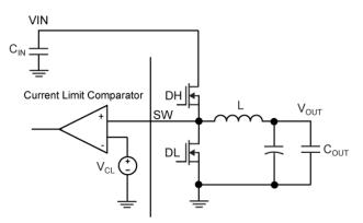
Figure 4. MIC2166 Current Limiting Circuit
