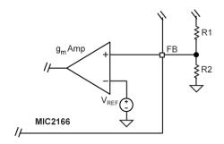
Figure 8. Voltage-Divider Configuration
