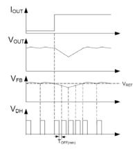
Figure 3. MIC2166 Load-Transient Response
