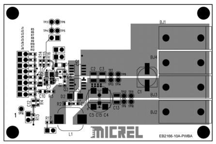
Figure 11. MIC2166 10A Evaluation Board Top Layer
