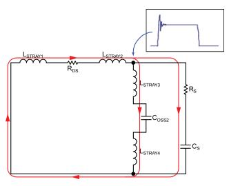
Figure 6. Snubber Circuit
