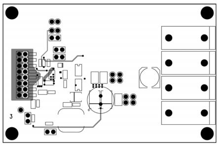
Figure 14. MIC2166 10A Evaluation Board Mid-Layer 2
