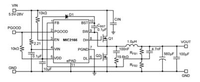
MIC2166 Adjustable Output 600kHz Buck Converter
