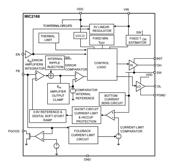
Figure 1. MIC2166 Block Diagram
