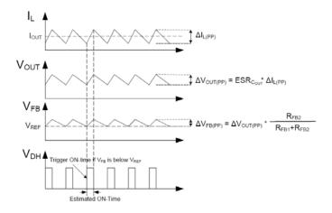
Figure 2. MIC2166 Control Loop Timing
