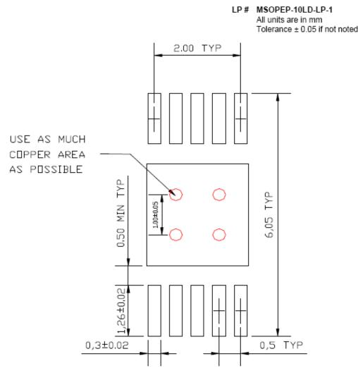
Red circle indicates Thermal Via. Size should be .300-.350 mm in diameter, 1.00 mm pitch, and it should be connected to GND plane for maximum thermal performance.
