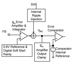
Figure 9. Internal Ripple Injection
