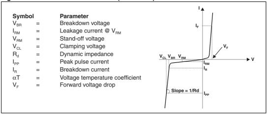
Table 2. Electrical characteristics ( $T_{amb} = 25$  °C)
