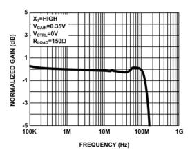
FIGURE 2. GAIN vs FREQUENCY ALL CHANNELS
