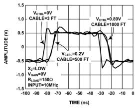
FIGURE 22. PULSE RESPONSE FOR VARIOUS CABLE LENGTHS
