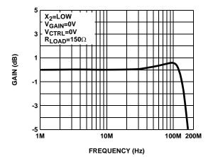
FIGURE 1. FREQUENCY RESPONSE OF ALL CHANNELS
