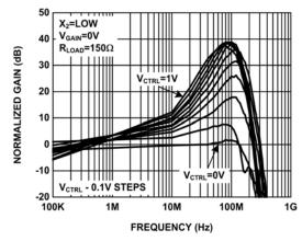
FIGURE 3. GAIN vs FREQUENCY FOR VARIOUS VCTRL
