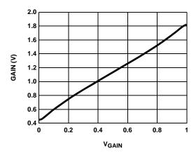
FIGURE 26. VARIATION OF GAIN WITH GAIN CONTROL VOLTAGE
