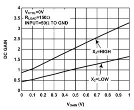
FIGURE 10. DC GAIN vs VGAIN
