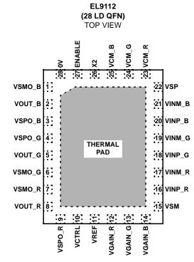
**EXPOSED DIEPLATE SHOULD BE CONNECTED TO -5V**
