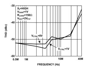
FIGURE 23. TOTAL HARMONIC DISTORTION
