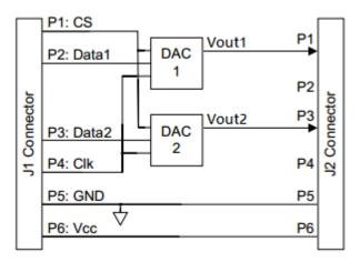
Figure 2. PmodDA2 circuit diagram.
