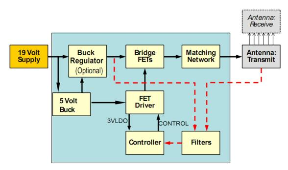
19 Volt Supply - the external 'brick' that converts AC power to 19 volts
