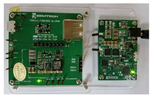
Connect a DC voltmeter across the VOUT+ and GND pins to monitor the voltage being output to the load, and a DC ammeter in series with the VOUT+ line. Set levels to allow for up to 10 volts and 3 amps to be observed.
