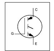
600 V  $I_{C(nom)} = 12 \text{A}$   $V_{CE(on)} \text{ typ.} = 1.55 \text{V} @$   $I_{C(nom)} @ 25 ^{\circ}\text{C}$ Motor Control IGBT
