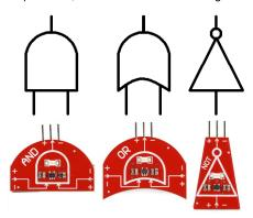
Each gate has one **output**, a male header (the pointy one). The female headers represent the **inputs**; the AND and OR gates have two inputs, while the NOT gate has just one.
