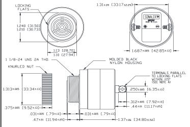
NOTE A: TERMINALS-032 BRASS TIN PLATED, TAPPED FOR #6-32 SCREW. TWO #6-32 NICKEL PLATED BRASS SCREWS INCLUBED. WILL ACCEPT 1/4' QUICK CONNECT. NOTE B: MOUNTING- REMOVE BLACK PLASTIC NUT AND INSERT THREADED FRONT THROUGH 1.25' HOLE PUNCHED IN PANEL, IF DRIENTATION IS NEEDED, NOTE LOCKING FLATS ON DRAWING. SCREW NUT BACK ON. DO NOT OVERTIGHTEN.
