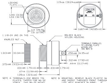
NOTE A: TERMINALS-032 BRASS TIN PLATED, TAPPED FOR #6-32 SCREW, TVD #6-32 NICKEL PLATED BRASS SCREWS INCLUDED, WILL ACCEPT 1/4' QUICK CONNECT.
