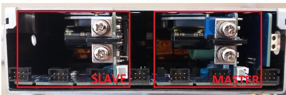
Since all Coolmod signals are isolated from the Coolmod outputs, when CoolMods are connected in series or parallel, all CoolMod analog control functions (Vtrim, Itrim, Enable/Inhibit) can be implemented by paralleling the appropriate signal pins of each CoolMod and providing a single control signal, i.e. connect all the Vtrim pins together and control Vtrim using a single control voltage. This can also be implemented using the PMBus™ interface.
