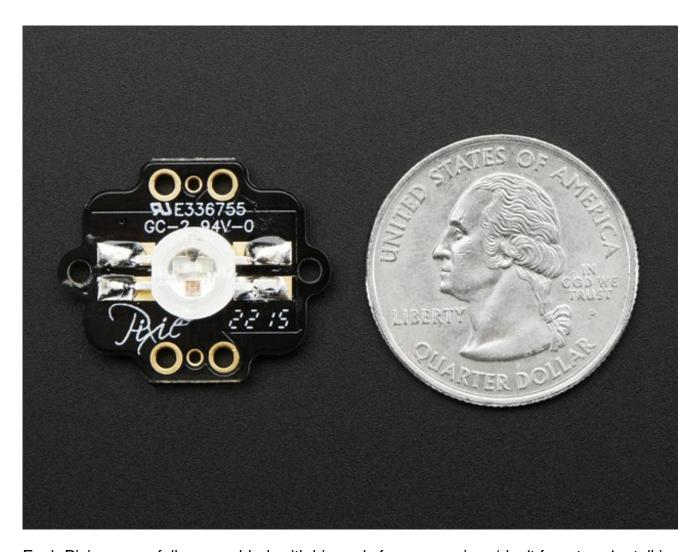
Each Pixie comes fully assembled, with big pads for power wires (don't forget, we're talking about max 1 Amp per Pixie!) and mounting holes on the sides. You'll also need thick wires to power each Pixie and a microcontroller that can send 115,200 baud 8N1 data to the Pixie (on its own, it will not do anything, you must send it data for it to light up)
