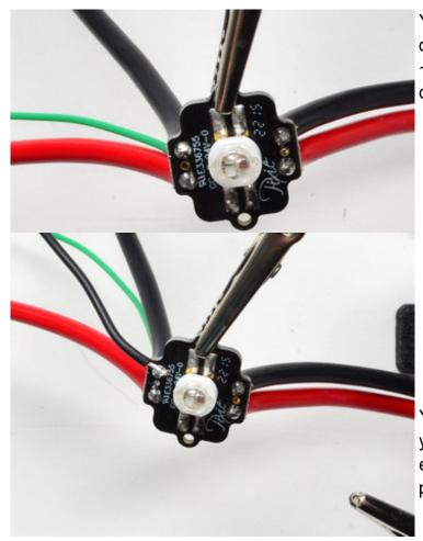
You can use a thinner wire for data, in this case we have a ~22AWG data line. It's soldered onto the **out** pin here
