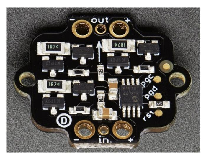
Pixie has two 'ports' - one for input and one for output. Both input and output ports have power pins:
