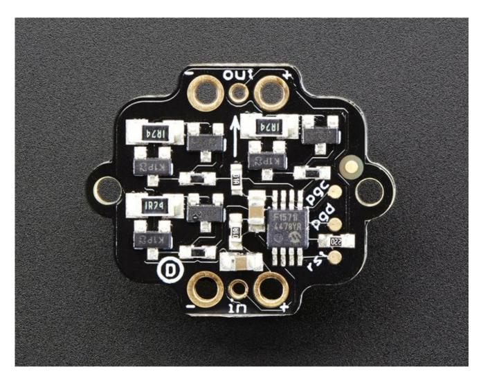
Since the Pixie uses so much power, there's a risk of the LED heating up so much it damages itself and/or the microcontroller. That's why Ytai added a temperature cut-off. When the PIC detects that the Pixie's temperature is too high, it turns off the LED until it gets back down to a reasonable level.
