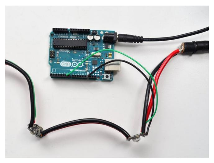
Wiring is easy, you can use any pin with a Serial or Software Serial output pin. We don't use the input of a Serial connection (since the Pixie is 'write only'). Dont forget to power the Pixie with a good 5V supply that can handle the current draw.
