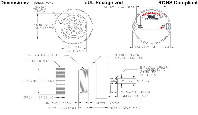
NOTE A: TERMINALS-.032 BRASS TIN PLATED, TAPPED FOR #6-32 SCREW. TWO #6-32 NICKEL PLATED BRASS SCREWS INCLUDED. WILL ACCEPT 1/4" QUICK CONNECT.
