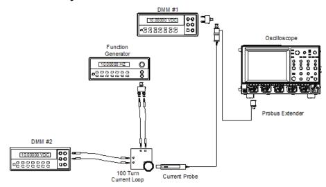
Figure 1. LF Accuracy Test set up.
