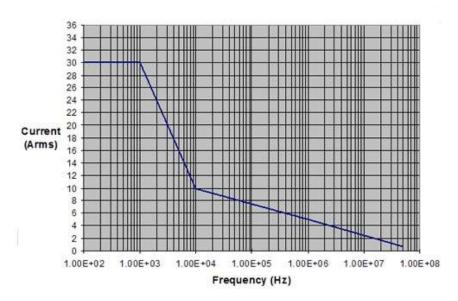
Figure 3. Maximum input current vs. frequency.
