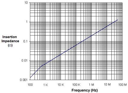
Figure 4. Insertion impedance vs. frequency.
