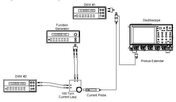
Figure 2. LF accuracy adjustment set up.
